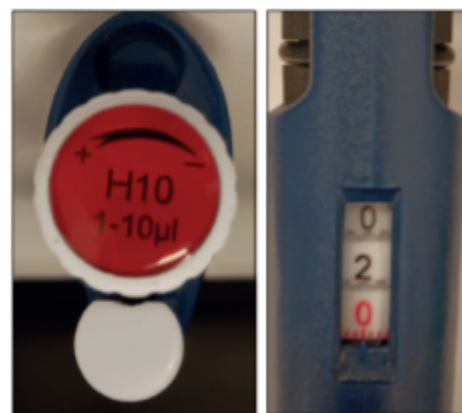
Example of a 1-10 µl micropipette set to 2 µl
