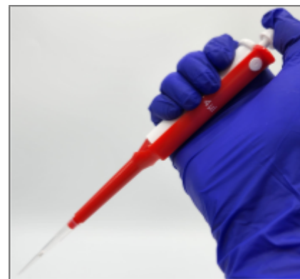
Example of 4 µl minipette with a 20 µl filter tip
