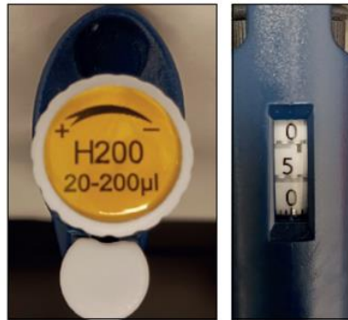
Example of a 20-200 \mu l micropipette set to 50 \mu l
