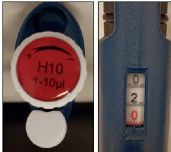
Example of a 1-10 \mu l micropipette set to 2 \mu l
