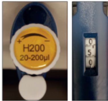
Example of a 20-200 µl micropipette set to 50 µl
