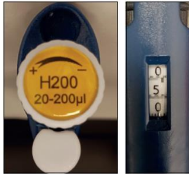
Example of a 20-200 µl micropipette set to 50 µl
