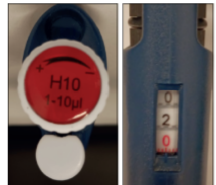
Example of a 1-10 µl micropipette set to 2 µl
