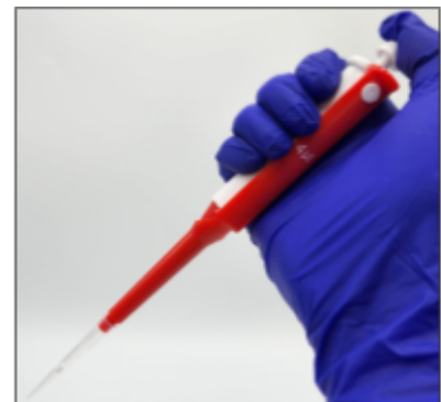
Example of 4 \mu l minipette with a 20 \mu l filter tip
