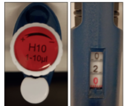
Example of a 1-10 \mu l micropipette set to 2 \mu l
